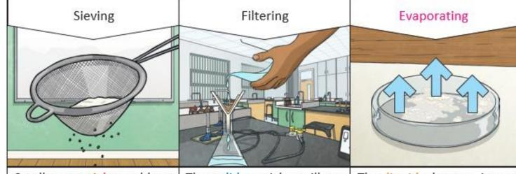
Smaller materials are able to fall through the holes in the sieve, separating them from larger particles.
